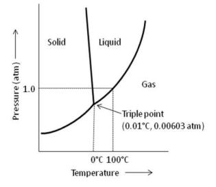
Figure 1 Phase diagram showing the triple point of water at 0.01°C, 0.00603 atm. Lyophilization is carried out below the triple point to enable conversion of ice into vapor, without entering the liquid phase (known as sublimation).
