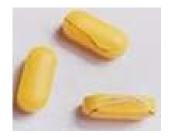
Figure 2 Cracks in the film created during the coating process.
