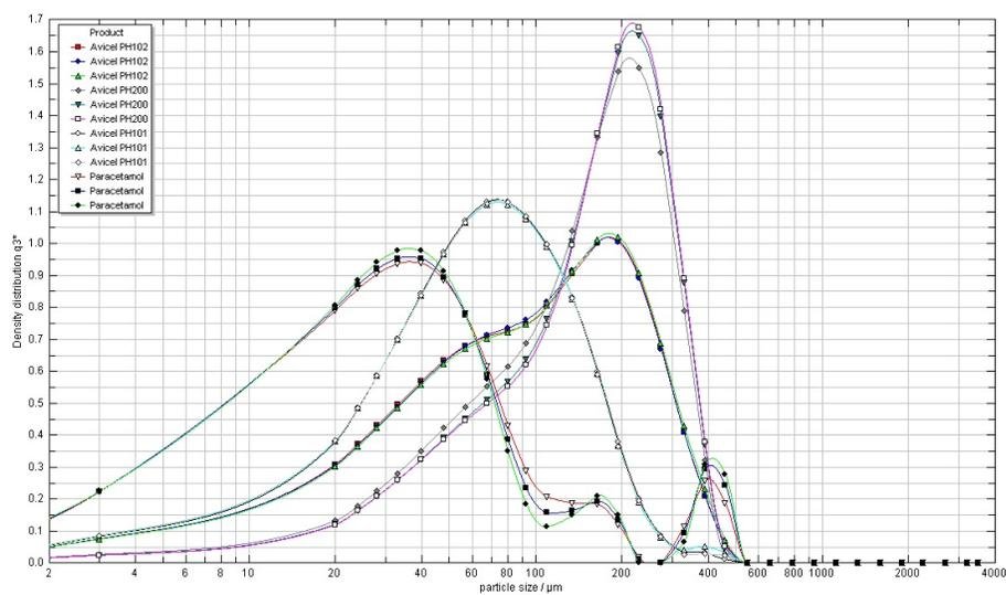
**Figure 5** The particle size distribution of paracetamol, Avicel PH101, PH102 and PH200.
