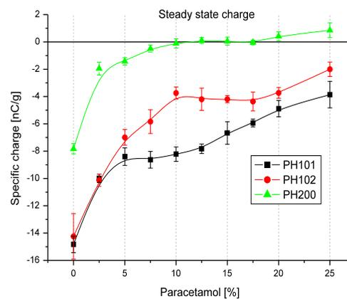
**Figure 7** Specific charge of different binary mixtures of MCC and paracetamol as a function of paracetamol concentration.
