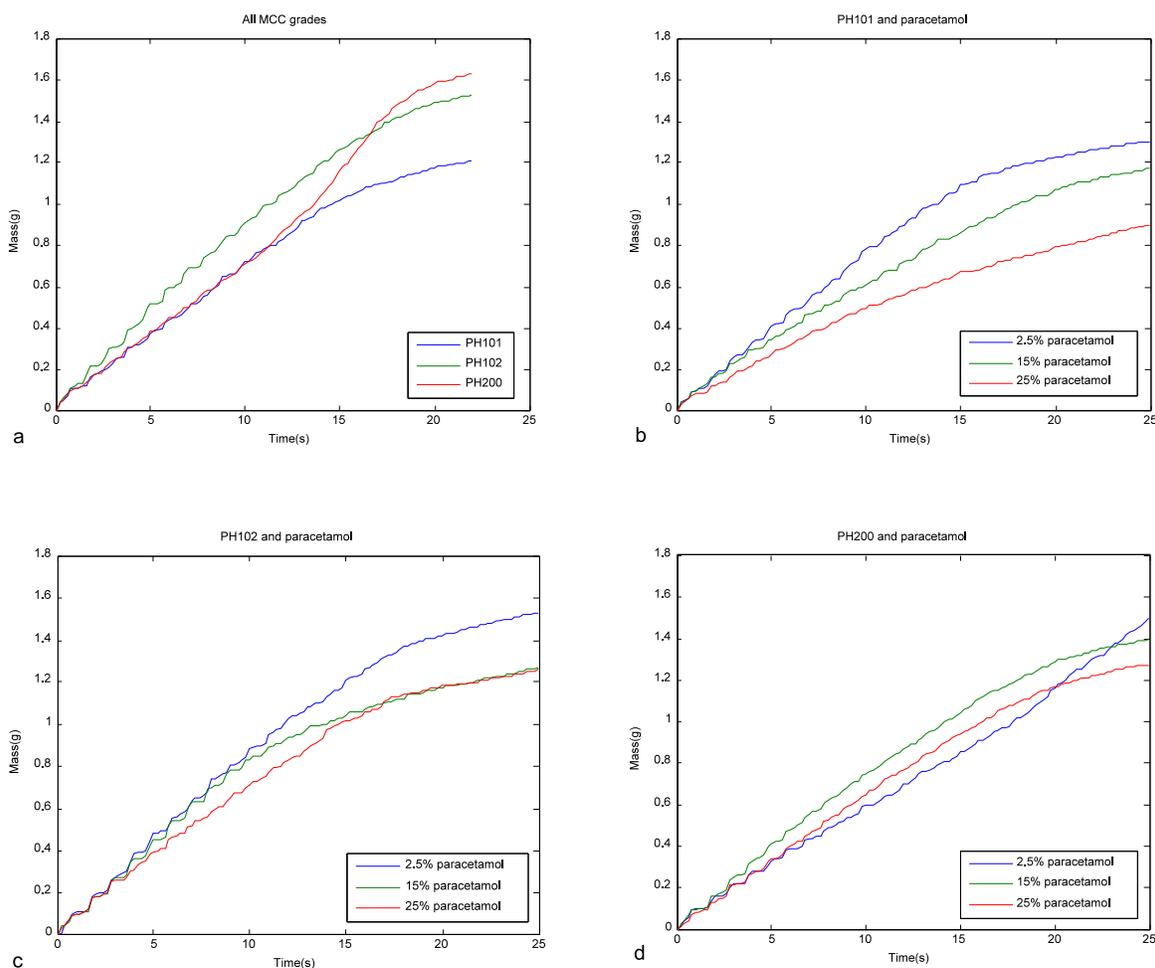
**Figure 2a-d** The effect of MCC grade (a) and different concentrations of paracetamol (b-d) on the flow rate of binary mixtures of paracetamol and MCC. The plots show the average of five measurements (relative standard deviation of most samples is below 6% and of all samples below 13%).
