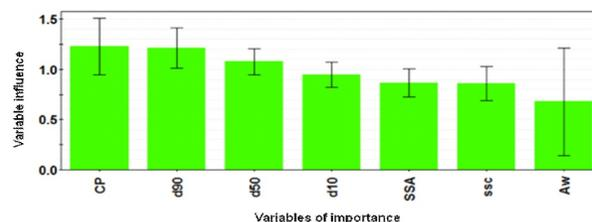
**Figure 9** Variables of importance (VIP) plot of the PLS model for prediction of powder flow. Terms with large VIP, larger than 1, are the most relevant for explaining Y (flow).
