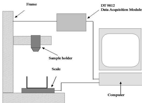
**Figure 1** A diagram of the flow measuring instrument and the experimental set-up.
