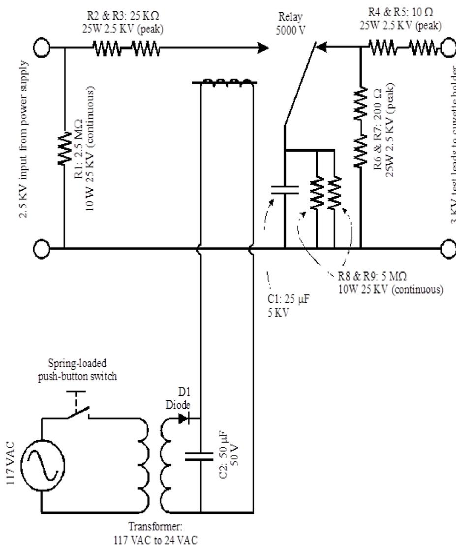
**Figure 2** Circuit diagram of an electroporation apparatus, as downloaded from the website <http://ebookbrowse.com/electroporator-doc-d25770175>. (The website does not have a digital object identifier (DOI) associated with it hence there is no guarantee that the link will be active in the future.)
