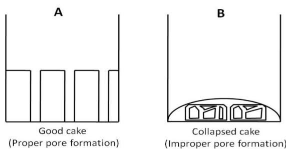
**Figure 7** Good cake structure ensures proper pore formation which provides the channels for vapor removal (A) whereas in case of cake collapse, a poor structure is obtained, leading to increased resistance in removal of vapor (B).
