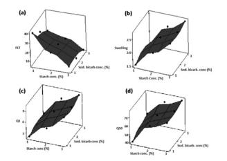
**Figure 4** Surface graphs showing effect of variables on (a), floating lag time, (b) swelling, (c) percent drug released in 1 hour  $(Q_1)$  and percent drug released in 10 hours  $(Q_{10})$ .
