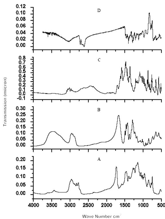
**Figure 1** ATR-FTIR Spectra: A: Eudragit E100; B: PVP; C: CPM; D: E 100:PVP:CPM matrix patch.
