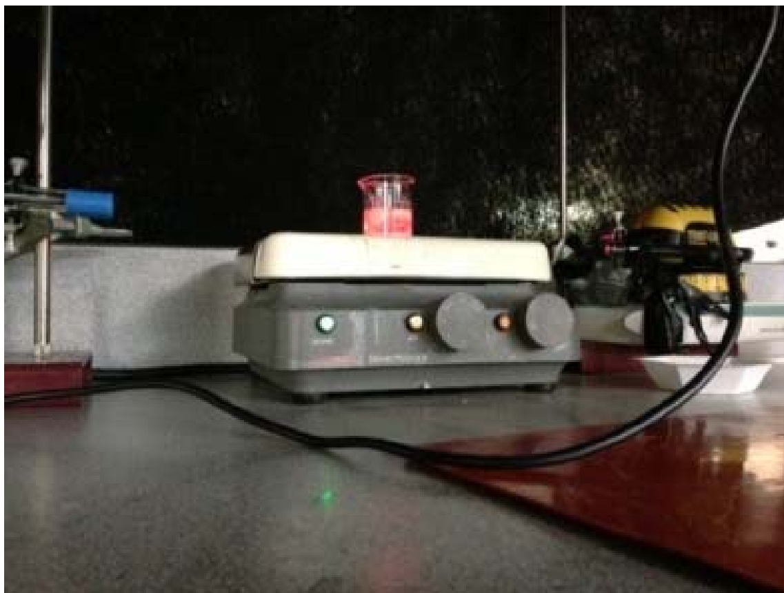
Figure 1 A sample of albumen during heating (Note: the light blocking assembly has been removed to show the details of the equipment set up)
